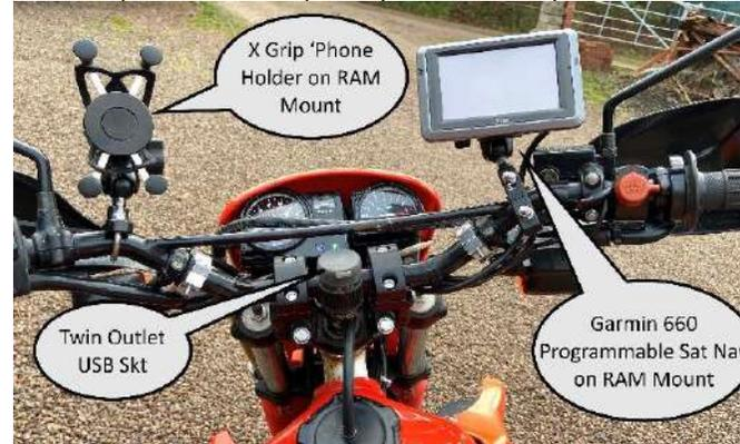
This is my chosen layout for Honda MTX 125 'Cockpit' with Garmin 660 Satnav, Smartphone X Grip holder and twin outlet USB socket for power to Smartphone or other accessories. 'Hardwired' on a fused homemade loom direct to the Bike Battery. **The assumption is that your bike will have 12 volt electrics. We will cover how to make this work on a 6 volt machine later in the series.**
