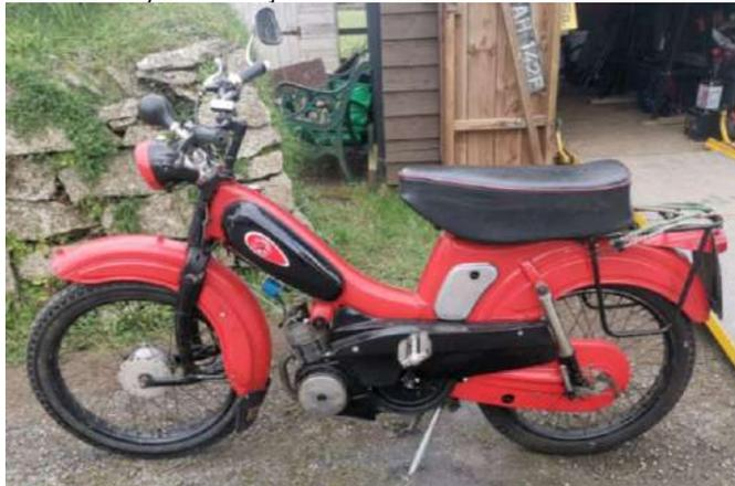
Made in the UK between 1961 and 1969, the RM5 was powered by a 49cc two-stroke engine with an automatic centrifugal clutch. These handsome mopeds with their leading link forks could manage 30 mph on a good day with a following wind.
