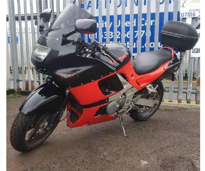
Outshone in the Sports/Tourer sector by the Yamaha 600s of the period, these 6 speed 4 cylinder ZZR600s are still top quality machines with 87hp at the rear wheel and 150+ mph top speed. Weighing just less than 200 kg, they are not too heavy to handle both on the road and in the garage. A functional fairing, fully adjustable suspension front and rear, plus twin 4-pot callipers add up to an excellent package. You can buy this one for £950.
