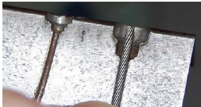
In use the cable is positioned in one side of the tool
