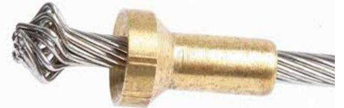
If you're making your own control cables, it is vital that you ensure that the inner cable cannot slip
