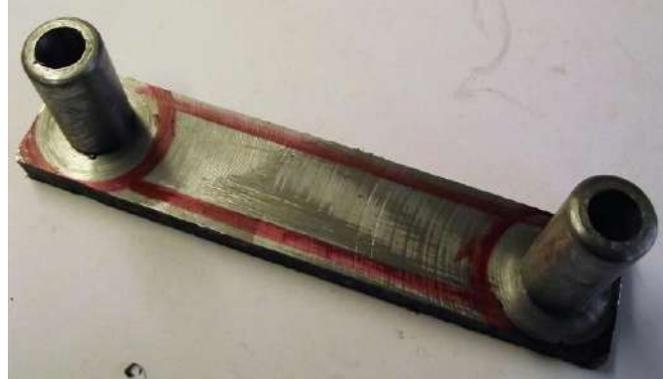
Screw spigots into side plates and assemble with steering stem and fork blades. All seems well with no play and free movement. Braze spigots into sideplates. Grind/file/linish links and with a coat of paint who would know they're homemade!! – **Thursday** - Nice and sunny outside of the shed so it's off for a pootle about on "Chuffa". (Sensible man Ed)
